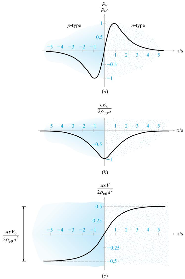
**Figure 6.12** (a) The charge density, (b) the electric field intensity, and (c) the potential are plotted for a  $pn$  junction as functions of distance from the center of the junction. The  $p$ -type material is on the left, and the  $n$ -type is on the right.
