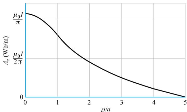
**Figure 7.20** The vector magnetic potential is shown within the inner conductor and in the region between conductors for a coaxial cable with  $b = 5a$  carrying  $I$  in the  $\mathbf{a}_z$  direction.  $A_z = 0$  is arbitrarily selected at  $\rho = b$ .
