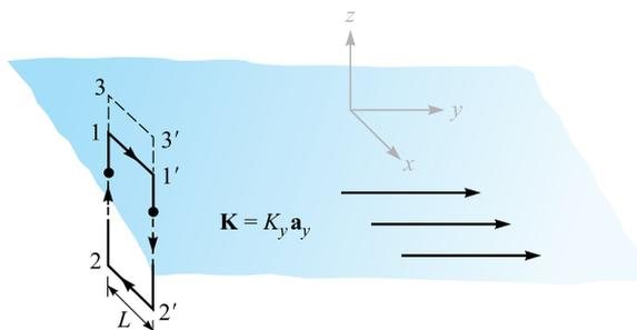
**Figure 7.10** A uniform sheet of surface current  $\mathbf{K} = K_y \mathbf{a}_y$  in the  $z = 0$  plane.  $\mathbf{H}$  may be found by applying Ampère’s circuital law about the paths 1-1'-2'-2-1 and 3-3'-2'-2-3.
