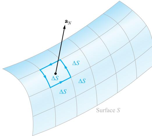
**Figure 7.16** The sum of the closed line integrals about the perimeter of every  $\Delta S$  is the same as the closed line integral about the perimeter of  $S$  because of cancellation on every interior path.
