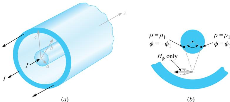
**Figure 7.8** (a) Cross section of a coaxial cable carrying a uniformly distributed current  $I$  in the inner conductor and  $-I$  in the outer conductor. The magnetic field at any point is most easily determined by applying Ampère's circuital law about a circular path. (b) Current filaments at  $\rho = \rho_1, \phi = \pm\phi_1$ , produces  $H_\rho$  components which cancel. For the total field,  $\mathbf{H} = H_\phi \mathbf{a}_\phi$ .
