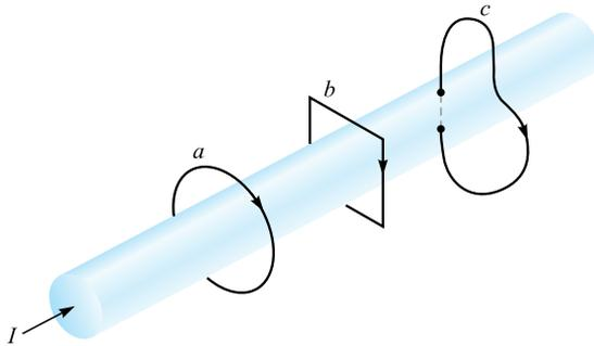
**Figure 7.7** A conductor has a total current  $I$ . The line integral of  $\mathbf{H}$  about the closed paths  $a$  and  $b$  is equal to  $I$ , and the integral around path  $c$  is less than  $I$ , since the entire current is not enclosed by the path.
