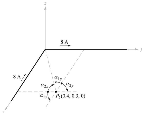
**Figure 7.6** The individual fields of two semi-infinite current segments are found by (9) and added to obtain  $\mathbf{H}_2$  at  $P_2$ .
