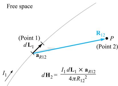
**Figure 7.1** The law of Biot-Savart expresses the magnetic field intensity  $d\mathbf{H}_2$  produced by a differential current element  $I_1 d\mathbf{L}_1$ . The direction of  $d\mathbf{H}_2$  is into the page.
