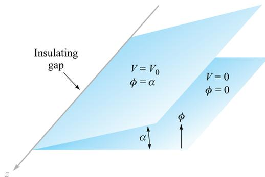
**Figure 6.10** Two infinite radial planes with an interior angle  $\alpha$ . An infinitesimal insulating gap exists at  $\rho = 0$ . The potential field may be found by applying Laplace's equation in cylindrical coordinates.
